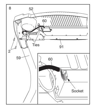
Insert the excess Wire Harness (60) into the large hole in the side of the Right Handrail (59). Securely tighten the plastic ties on the bottom of the Console Base (52) to prevent the Wire Harness from slipping. Then, cut off the ends of the plastic ties.
